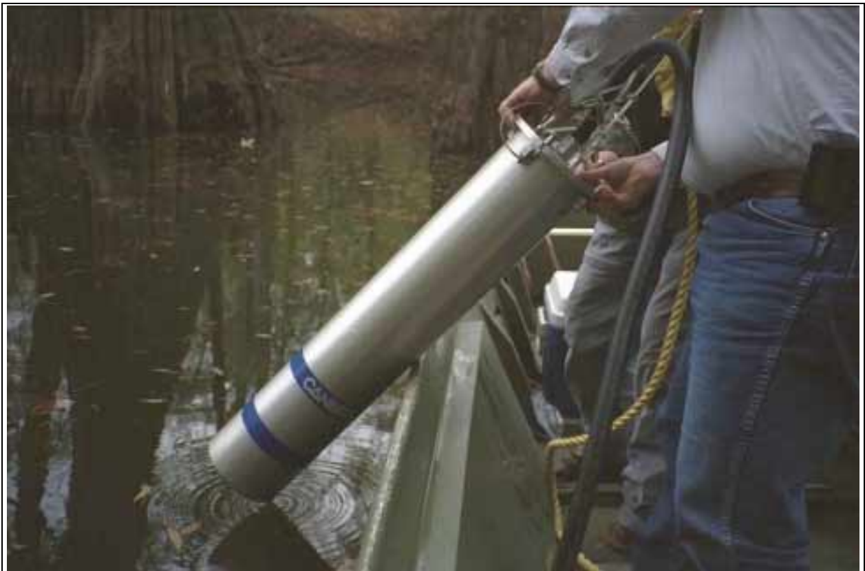
Figure B-11: Underwater Gamma Spectrometer for testing the bottom of the Savannah River
