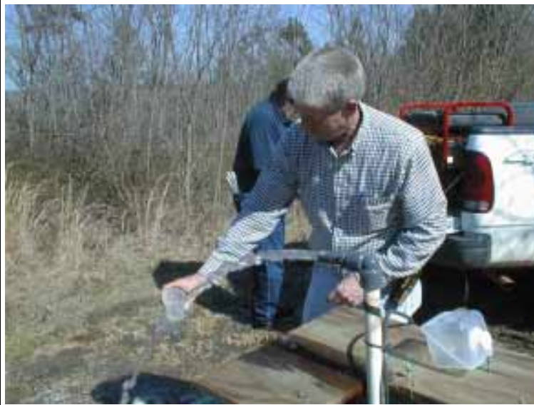
Figure B-4 Underflow Study Groundwater Sampling by EPD and SRS Personnel
