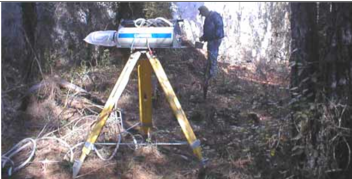
Figure I-1: Monitoring for Gamma Radiation Outside of the Hot Cell Building at DFWMA
