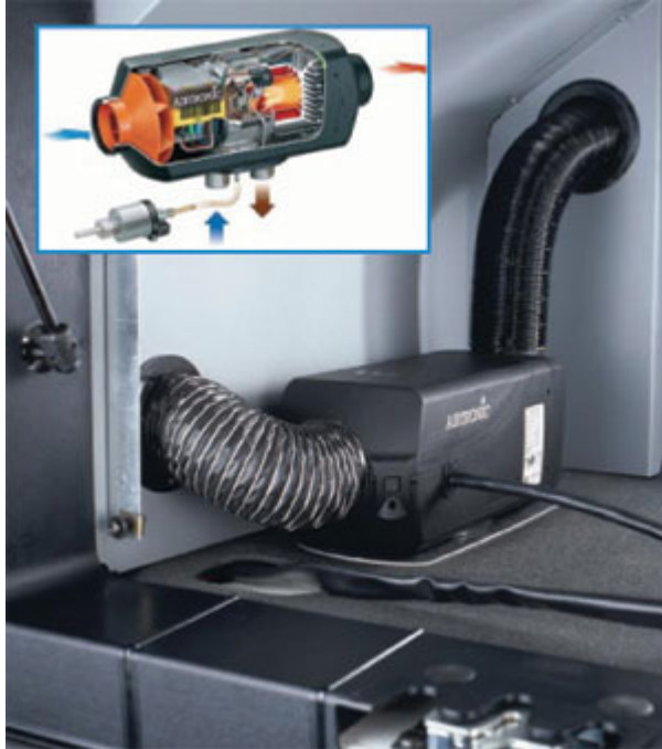
Figure 2.5.3. The above picture shows a diesel heating system.
