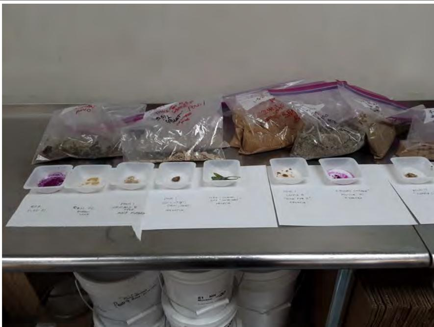
Photo 2: Sequence of first 8 tests with controls - JEA Ash (far left), 5 Pond 1 soil samples, crushed concrete and Pond 1 soil
